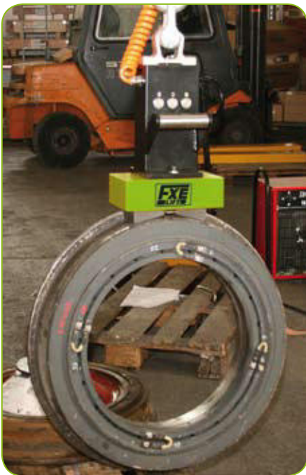
FXE with pole shoe for railway wheels
