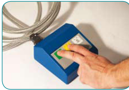
Step 2: Activating the Magnetic Chuck
