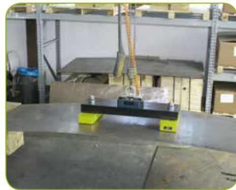
FXE-T to move thin sheet
